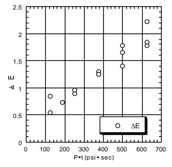
Figure 2. Color Transfer at 60°C versus the Pressure Time Product
