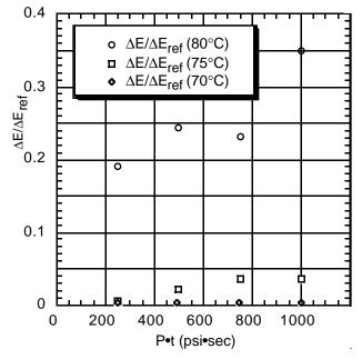
Figure 4. Temperature Dependence of Blocking Transfer in Color Laser Toner Prints
