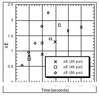
Figure 1. Color Transfer versus Time at Various Pressures (T = 60 °C).
